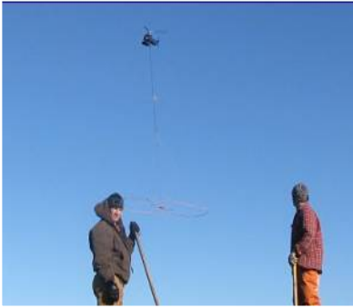
Helicopter Airborne VTEM Survey St. Juliens 2008
